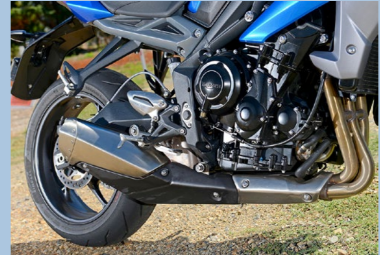
Engine is straight from the Daytona 675, and there's also the new low slung exhaust for 2013.
