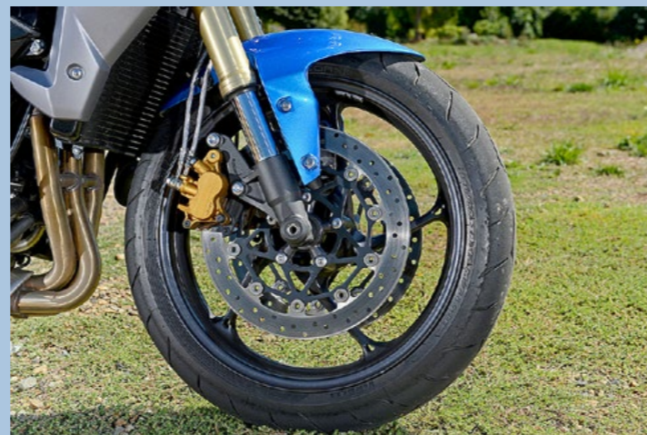
Two-piston Nissin calipers work a treat.
