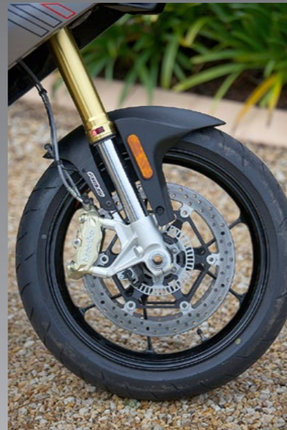
Forks have dynamic damping too, and the massive Brembos of course.
