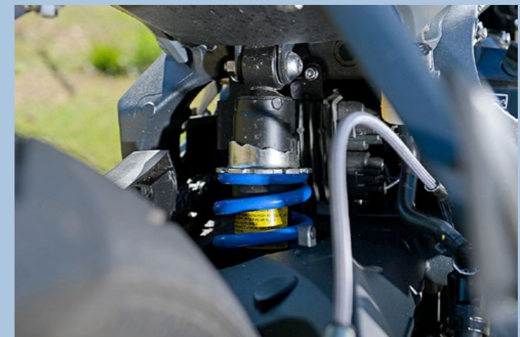
Rear shock has preload adjustment.
